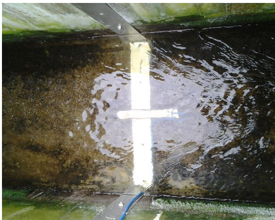
Multi-correlation doppler sensor installation
