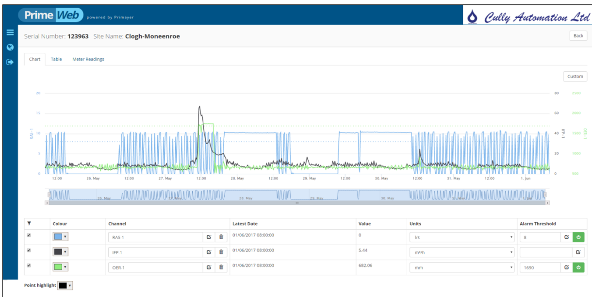
PrimeWeb data chart enabling operator analysis of XiLog flow and depth readings
