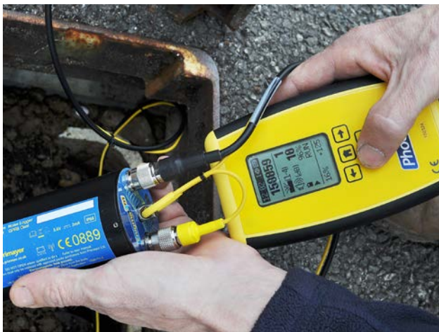
Programming with Comms Module.
