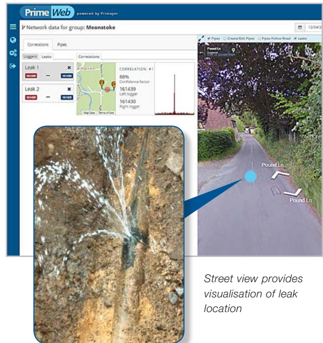
Correlation function displayed with frequency spectrum and coherence.
