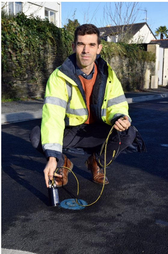
Leak technician about to install an Enigma3m logger
