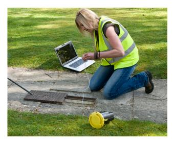
The flow input can log two uni-directional flows or one bi-directional flow. Also, both outputs from combination meters can be logged on one logger input channel. Existing meter index value can be entered at start of logging.
