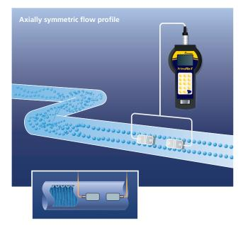
Correct positioning of the sensors is crucial to collect accurate data
