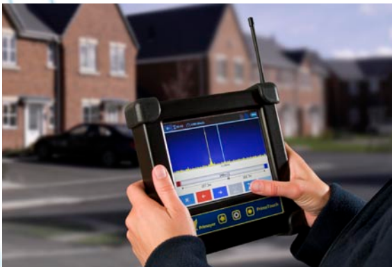
Clear correlation display of leak position
