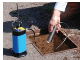
Use of separate accelerometer
